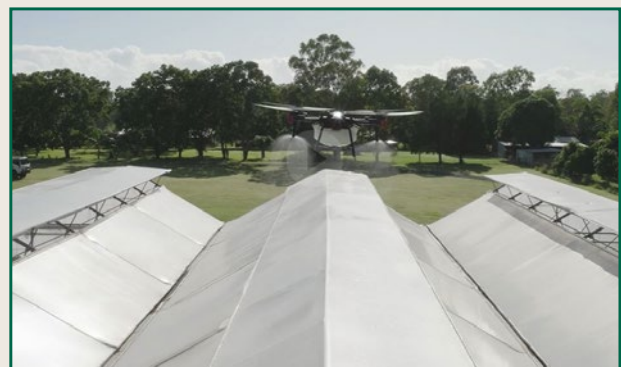
FIGURE 8: Drone Applying Whitewash to Greenhouse Covers
